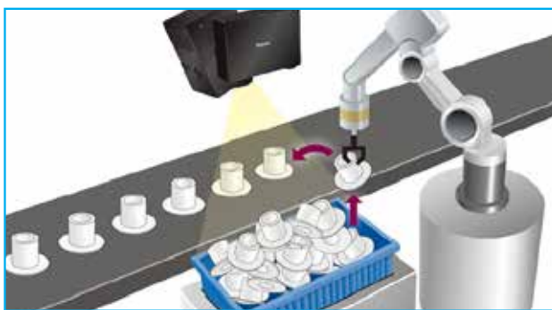
Inspection: Inspect for assembly errors, surface defects, damaged parts and missing features. Identify the orientation, shape and position of objects and features
