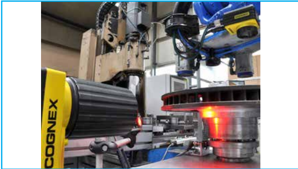
Automotive: In-Sight vision systems critical to successful handling and character reading of turned parts
