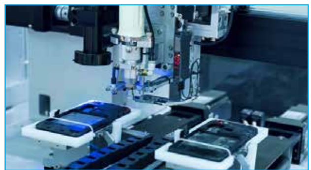
Guide/Align: Guide automation equipment and robotic devices. Align parts for high accuracy assembly operations and other manufacturing processes.
