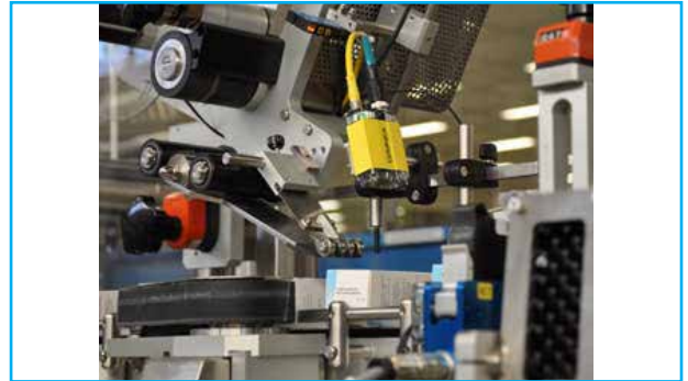
Pharmaceutical Distributors: Track and trace of pharmaceutical folding boxes with Cognex vision systems: certain to be original
