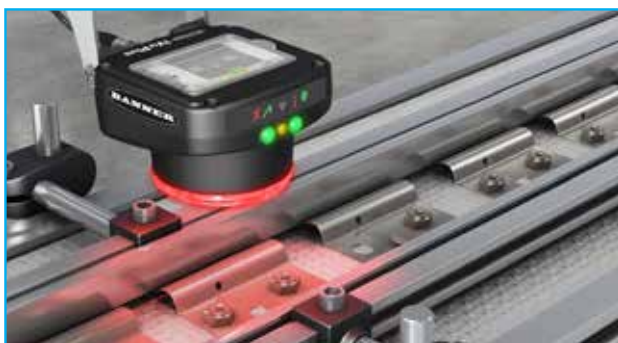
Presence/Absence: Detect the presence or absence of simple features and objects to give basic pass/fail results.
