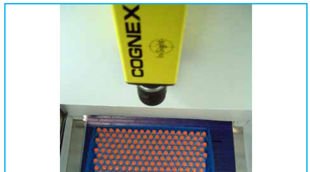
Medical Devices: Vision system eliminates count deviations, inspects vials
