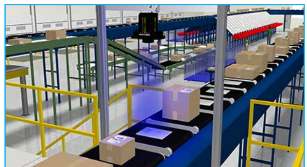
Code Reading: Read 1-D barcodes and 2-D matrix codes as part of an overall inspection.
