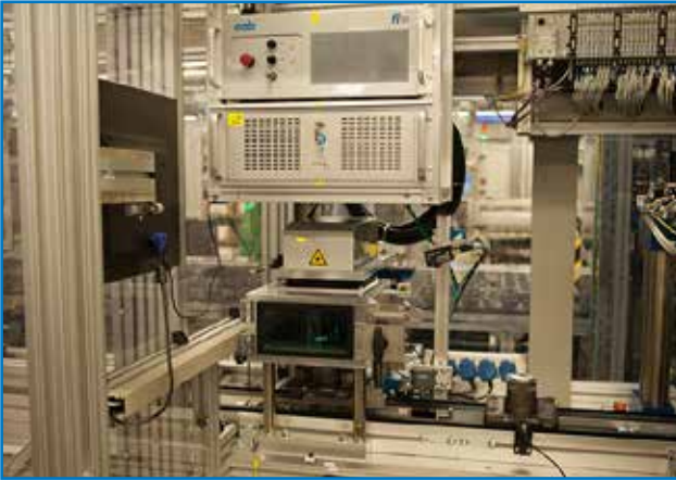
Auto: ZF TRW uses fiber lasers to encode gas generators of airbags.
