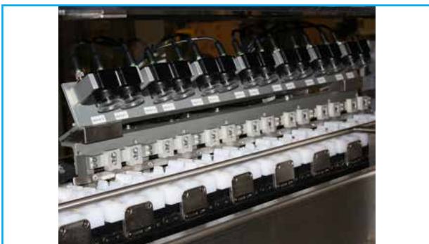
Food and Beverage: Vision Sensor Helps Automate High-Speed Loading of Transparent Cartons
